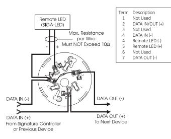
Isolator Detector Base, SIGA-IB, SIGA-IB4
